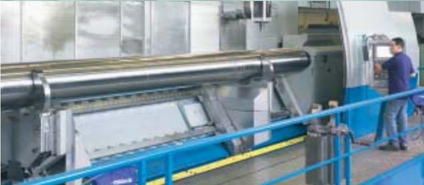
Finish machining of a bimetallic barrel
